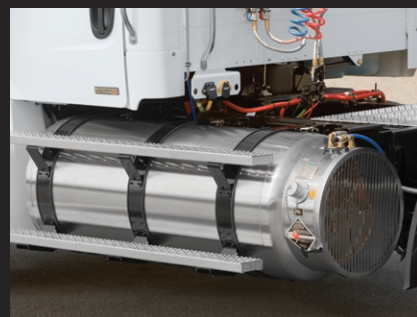
Stainless steel LNG fuel tanks are designed to keep fuel in its liquid state and offer an approximate range of 440 miles depending on your application.
