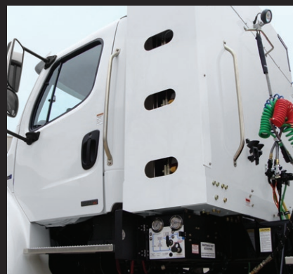
Housed in an enclosure behind the cab, carbon fiber reinforced aluminum type 3 compressed natural gas (CNG) fuel tanks offer an approximate range of 400 miles depending on your application.
