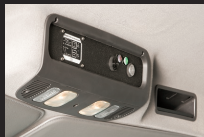
Standard methane gas detection system alerts the driver in the event of a fuel leak.
