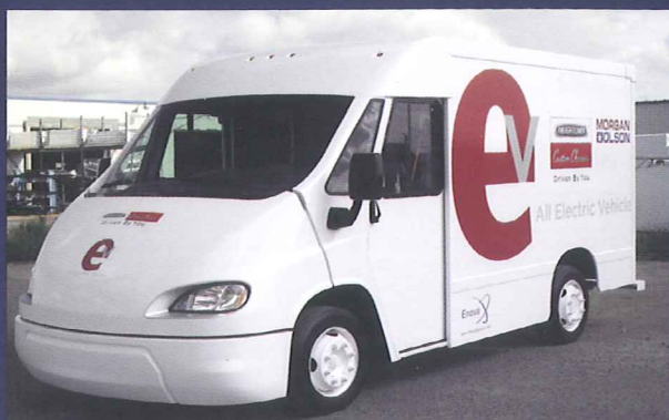
FCCC Walk-in Van Chassis With all-electric drive system
